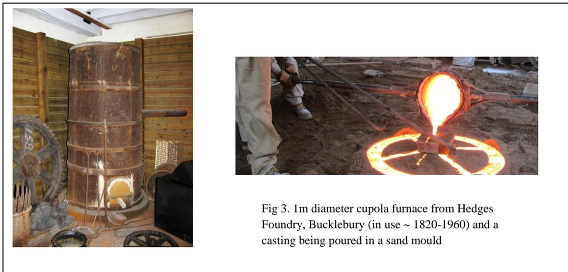
Fig 3. 1m diameter cupola furnace from Hedges Foundry, Bucklebury (in use ~ 1820-1960) and a casting being poured in a sand mould
