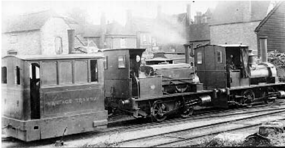
Wantage Tramway - c1900? - Matthews No.6 box engine, Manning-Wardle engine No.7, and George England engine No.5 in Wantage top yard. Car 3? in background. Note the track construction: longitudinal baulks and cross-ties. (tr138.jpg)
